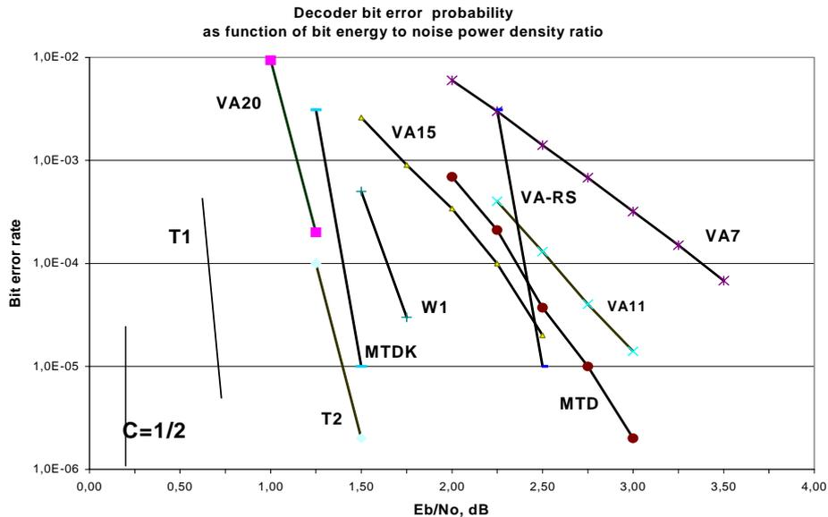
gives. The best turbo code with  $R=1/2$  and the length code  $n=130'000$  bits is presented with line T1 [6], cascaded "woven" code with  $n=2000$  bits - curve W1 [7], and turbo code of length 3570 [8] - curve T2.
