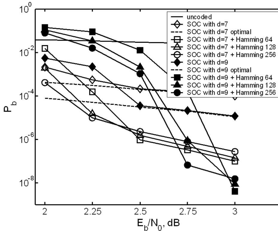
Fig. 2. Performance of the concatenated coding scheme, consisting of SOC with code rate 1/2 and Hamming code, over AWGN channel
