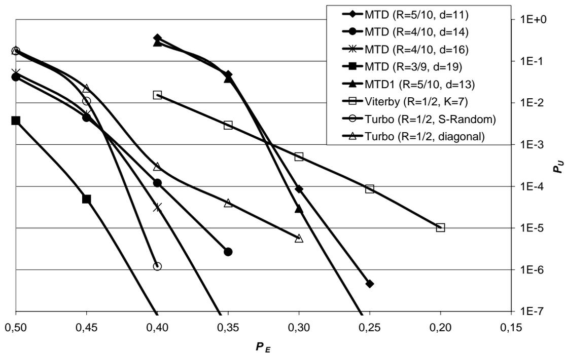
Fig. 2. Performance of MTD over the channel with erasures and errors
